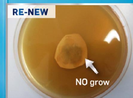
„Real life“ application test: elimination of moulds by covering
